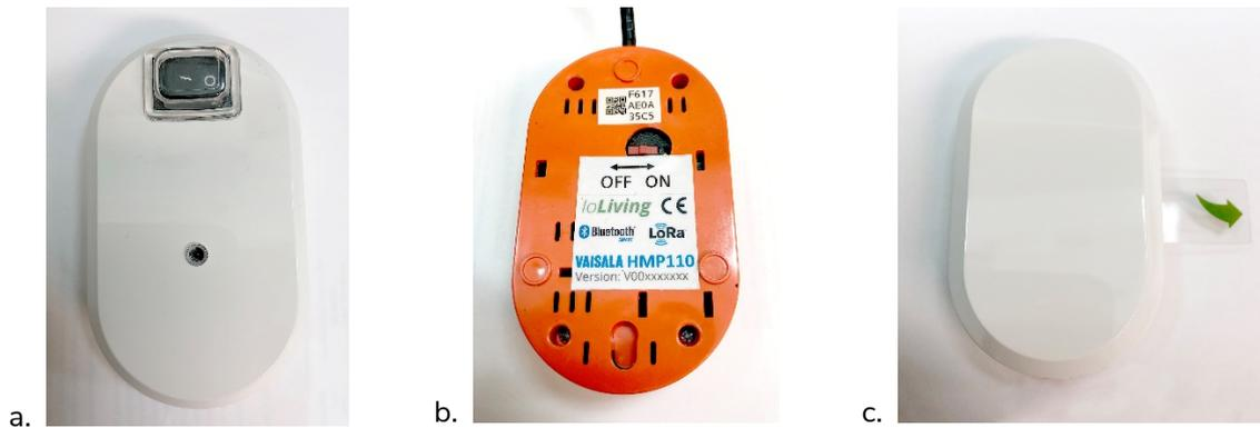
Figure 1. The power switch type can be (a) rocker switch, (b) slider switch or (c) battery strip which must be removed by pulling it straight out.
